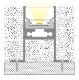
The strip is attached to the aluminium guide for precise and quick insertion
